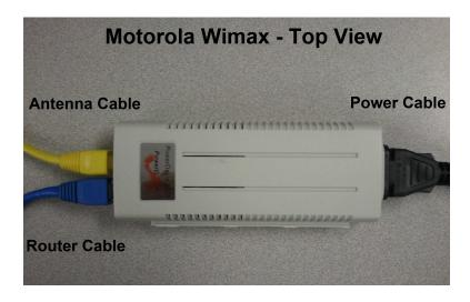
If the internet is not working, try to unplug just the power cable from the off-white WiMAX power box(Never mess with the two Ethernet cables unless a technician instructs you to) for about 15 minutes and make sure both green lights comes back on solid. If internet still does not work try to power cycle your router and/or your computer.
