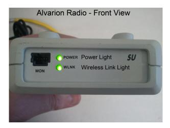
If neither the WLNK nor PWR lights are on, try to unplug the power from the Breeze Access box for at least 15 minutes. Once plugged back in, it takes the box approx. 45 seconds to fully boot up so the lights will blink during this time.
